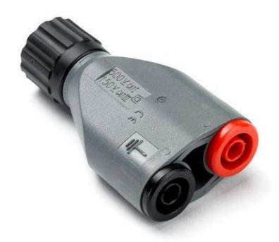
The BNC to 4 mm adapter connects two 4 mm ("banana") plugs to a BNC socket. If you have a sensor such as a current clamp with 4 mm plug outputs, for example, this adapter allows you to plug it into a PicoScope Automotive Oscilloscope with a BNC input. The 4 mm sockets and BNC plug are fully shrouded for safety.
