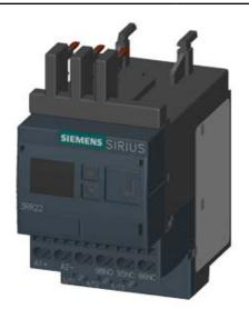
MONITORING RELAY ATTACHABLE TO CONTACTOR 3RT2. SIZE S0 STANDARD, DIGITAL ADJUSTABLE APPARENT/ACTIVE CURRENT MONIT. 4 - 40A, 20-400 HZ, 3-PHASE SUPPLY 24-240 V AC/DC 1 CO CONTACT, 1 SEMICOND. FOR ALARM AND WARNING MONITORING FOR CURRENT OVERSHOOT/UNDERSHOOT PHASE FAILURE, WIRE BREAK PHASE SEQUENCE FAULT CURRENT BLOCKING CURRENT WARNING AND ALARM THRESHOLDS WITH OR W/O ERROR LOG ONDELAY 0-99 S SPURIOUS PEAK SUPPR.0-30 S BREAK AFTER FAULT 0-300 MIN SCREW CONNECTION
