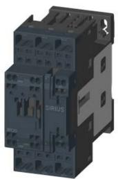
CONTACTOR, AC-3, 5.5KW/400V, 1NO+1NC, AC 230V 50HZ, 3-POLE, SZ S0 SPRING-LOADED TERMINAL
