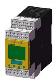
SIRIUS SAFETY RELAY SAFETY-RELATED SPEED MONITORING, 24 V DC, 45.0 MM, SCREW-TYPE CONNECTION, ENABLING CIRCUIT INSTANTANEOUS:2NO, ENABLING CIRCUIT DELAYED:0, SIGNALING CIRCUIT:2 ELECTRICAL, NAMUR VERSION AUTO START / MANUAL START, BASIC UNIT, MAX. ERR. PL EN13849-1: E, MAX. ERR. SIL TO IEC61508:3,
