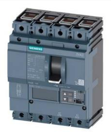
CIRCUIT BREAKER 3VA2 IEC FRAME 100 BREAKING CAPACITY CLASS M ICU=55KA @ 415 V 4POLE, LINE PROTECTION ETU550, LSI, IN=63A OVERLOAD PROTECTION IR=25A ...63A SHORT CIRCUIT PROTECTION ISD=0,6..10X IN, II=1,5..12X IN NEUTRAL PROTECTION ADJUSTABLE (OFF, UPTO 160%) CABLE CONNECTION
