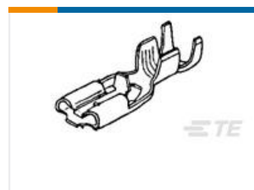
TE Part #170325-1 187 PL MKII REC. 20-16AWG PTBR
