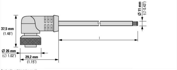
Supply cable, prefabricated on one side
