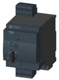
SIRIUS, COMPACT STARTER, REVERSING STARTER 690 V, 24 V AC/DC, 50 ... 60 HZ, 3 ... 12 A, IP20, MAIN CIRCUIT CONNECTION: SPRING-LOADED TERMINAL, AUXILIARY CIRCUIT CONNECTION: PLUG-IN, W/O TERMINALS
