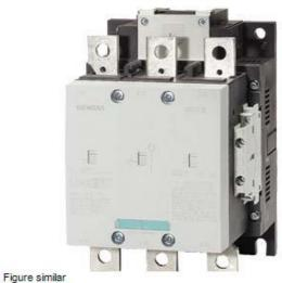
VAC. CONTACTOR, 160KW/400V/AC-3 AC(40...60HZ)/DC OPERATION UC 110-127V AUXILIARY CONTACTS 2NO+2NC 3-POLE, SIZE S10 BAR CONNECTIONS CONVENT. OPERATING MECHANISM
