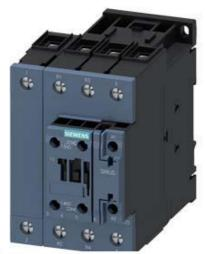
2NO+2NC CONTACTOR,AC3:18.5KW 83 - 155 V AC/DC, VARISTOR, 4-POLE, 2NO+2NC, SIZE S2, SCREW TERMINAL 1NO+1NC INTEGRATED
