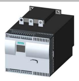
SIRIUS SOFT STARTER, VALUES WITH 460 V, 50 DEG., STANDARD: 100A, 75HP, INSIDE-DELTA CIRCUIT 3: 173A, 125HP, 200-460 V AC, 115 V AC, CAGE CLAMP TERMINALS
