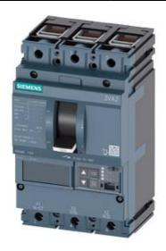
CIRCUIT BREAKER 3VA2 IEC FRAME 160 BREAKING CAPACITY CLASS H ICU=85KA @ 415 V 3POLE, LINE PROTECTION ETU550, LSI, IN=40A OVERLOAD PROTECTION IR=16A ...40A SHORT CIRCUIT PROTECTION ISD=0,6..10X IN, II=1,5..12X IN NEUTRAL PROTECTION OPTIONAL WITH EXT. CT,UPTO 160% CABLE CONNECTION
