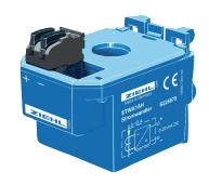
The STWA1AH is a measuring transducer for AC currents 0...15 A. Multiple loops of the conductor through the transformer reduces the measuring range correspondingly (for instance to 0...5 A with three loops).
