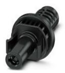
Photovoltaic connector, Range of articles: SUNCLIX, Photovoltaic connector, housing material: PPE, color: black, number of positions: 1, min. conductor cross section: 2.5 mm², max. conductor cross section: 6 mm², nom. voltage: 1500 V, rated current: 26 A, Connection method: Crimp, Type of contact: Socket
