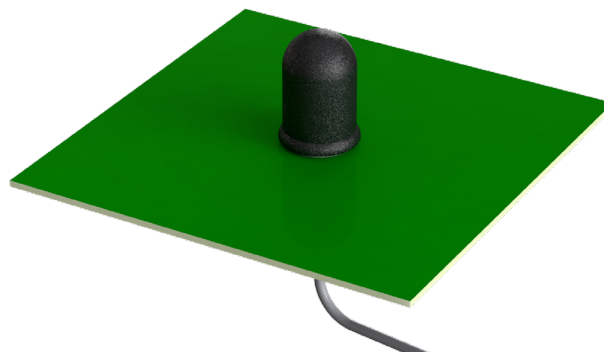
Figure 3. ANT-2.4-WRT-MON Test Orientation
