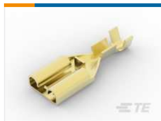
TE Model / Part # 63933-1 PL .250 TERMINAL REC 22-18 AWG BR
