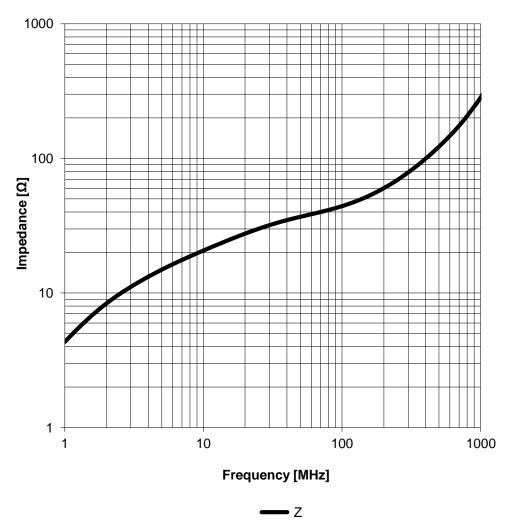
CHECKED GENERAL TOLERANCE PROJECTION METHOD CREATED Würth Elektronik eiSos GmbH & Co. KG EMC & Inductive Solutions KaS KaS DIN ISO 2768-1m Max-Eyth-Str. 1 74638 Waldenburg **WE-AFB EMI Suppression Axial** Tel. +49 (0) 79 42 945 - 0 **Ferrite Bead** ORDER CODE www.we-online.com 742700391 eiSos@we-online.com DATE (YYYY-MM-DD) BUSINESS UNIT REVISION STATUS PAGE 001.001 Valid 2/4 2018-02-20 eiSos **WÜRTH ELEKTRONİK**
