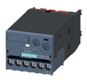
SOLID-STATE TIME RELAY ON-DELAY WITH SEMICONDUCTOR OUTPUT 24...240V AC/DC, TIME RANGE 0.05...100S, FOR SNAPPING ONTO THE FRONT, FOR 3RT2 CONTACTORS S00/S0 SCREW TERMINALS INTEGRATED VARISTOR FOR DAMPING CONTACTOR COILS
