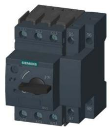
CIRCUIT-BREAKER SZ S0, FOR MOTOR PROTECTION, CLASS 10, W. OVERLOAD RELAY FUNCTION A-RELEASE18...25A, N-RELEASE 325 A, SCREW CONNECTION, STANDARD SW. CAPACITY
