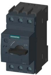
CIRCUIT-BREAKER SZ S0, FOR TRANSFORMER PROT. A-RELEASE 10...16A, N-RELEASE 286A, SCREW CONNECTION, STANDARD SW. CAPACITY
