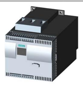
SIRIUS SOFT STARTER, VALUES WITH 460 V, 50 DEG., STANDARD: 82A, 60HP, INSIDE-DELTA CIRCUIT 3: 142A, 100HP, 200-460 V AC, 115 V AC, SCREW TERMINALS
