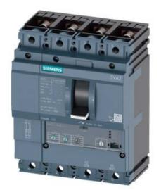
CIRCUIT BREAKER 3VA2 IEC FRAME 100 BREAKING CAPACITY CLASS C ICU=110KA @ 415 V 4POLE, LINE PROTECTION ETU320, LI, IN=40A OVERLOAD PROTECTION IR=16A ...40A SHORT CIRCUIT PROTECTION II=12 X IN NEUTRAL PROTECTION ADJUSTABLE(OFF,100%) BUSBAR CONNECTION
