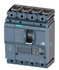
CIRCUIT BREAKER 3VA2 IEC FRAME 160 BREAKING CAPACITY CLASS C ICU=110KA @ 415 V 4POLE, LINE PROTECTION ETU550, LSI, IN=63A OVERLOAD PROTECTION IR=25A ...63A SHORT CIRCUIT PROTECTION ISD=0,6..10X IN, II=1,5..12X IN NEUTRAL PROTECTION ADJUSTABLE (OFF, UPTO 160%) CABLE CONNECTION
