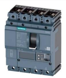
CIRCUIT BREAKER 3VA2 IEC FRAME 160 BREAKING CAPACITY CLASS C ICU=110KA @ 415 V 4POLE, LINE PROTECTION ETU860, LSIG, IN=63A OVERLOAD PROTECTION IR=25A ...63A SHORT CIRCUIT PROTECTION ISD=0,6..10X IN, II=1,5..12X IN NEUTRAL PROTECTION ADJUSTABLE (OFF, UPTO 160%) GROUNDFAULT, SWITCHABLE IG=0,2... 1 X IN, TG=0,050,8MS BUSBAR CONNECTION
