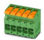
PCB terminal block, nominal current: 76 A, rated voltage (III/2): 1000 V, nominal cross section: 16 mm², Number of potentials: 5, Number of rows: 1, Number of positions per row: 5, product range: LPT 16/, pitch: 10 mm, connection method: Lever Push-in connection, mounting: Wave soldering, conductor/PCB connection direction: 0 °, color: green, Pin layout: Zigzag pinning W, Solder pin [P]: 3.6 mm, type of packaging: packed in cardboard
