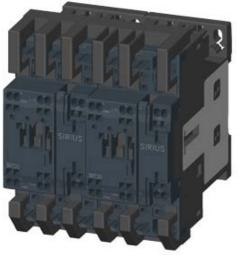
REV. COMB., AC3, 15KW/400V AC230V, 50/60HZ, 3-POLE, SZ S0 SPRING-LOADED TERMINAL ELECTR. AND MECH. INTERLOCK 2NO INTEGR.
