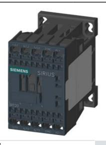
COUPLING RELAY, AC-3, 3KW/400V, 1NC, DC 24V, 0.85...1.85\*US, 3-POLE, SZ S00 SPRING-LOADED TERMINAL
