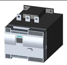
SIRIUS SOFT STARTER, VALUES WITH 575 V, 50 DEG., STANDARD: 215A, 200HP, INSIDE-DELTA CIRCUIT 3: 372A, 350HP, 400-690 V AC, 115 V AC, SCREW TERMINALS
