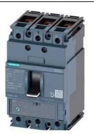
CIRCUIT BREAKER 3VA1 IEC FRAME 160 BREAKING CAPACITY CLASS M ICU=55KA @ 415 V 3-POLE, LINE PROTECTION TM220, ATFM, IN=100A OVERLOAD PROTECTION IR=70A ...100A SHORT CIRCUIT PROTECTION II=10 X IN BUSBAR CONNECTION
