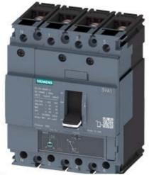
CIRCUIT BREAKER 3VA1 IEC FRAME 160 BREAKING CAPACITY CLASS M ICU=55KA @ 415 V 4-POLE, LINE PROTECTION TM220, ATFM, IN=100A OVERLOAD PROTECTION IR=70A ...100A SHORT CIRCUIT PROTECTION II=10 X IN NEUTRAL PROTECTION 100% BUSBAR CONNECTION
