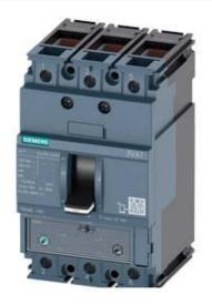
CIRCUIT BREAKER 3VA1 IEC FRAME 160 BREAKING CAPACITY CLASS H ICU=70KA @ 415 V 3-POLE, LINE PROTECTION TM240, ATAM, IN=63A OVERLOAD PROTECTION IR=44,1A ...63A SHORT CIRCUIT PROTECTION II=5...10 X IN CABLE CONNECTION
