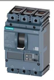
CIRCUIT BREAKER 3VA2 IEC FRAME 160 BREAKING CAPACITY CLASS C ICU=110KA @ 415 V 3POLE, LINE PROTECTION ETU860, LSIG, IN=25A OVERLOAD PROTECTION IR=10A ...25A SHORT CIRCUIT PROTECTION ISD=0,6..10X IN, II=1,5..12X IN NEUTRAL PROTECTION OPTIONAL WITH EXT. CT,UPTO 160% GROUNDFAULT, SWITCHABLE IG=0,2... 1 X IN, TG=0,050,8MS CABLE CONNECTION
