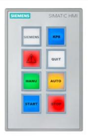
SIMATIC HMI KP8F PN, KEY PANEL, 8 SHORT-STROKE KEYS WITH MULTI-COLOR LED'S, PROFINET INTERFACE WITH PROFISAFE, 8 DI/DO AND 2 SAFETY DI PINS, 24V DC LOOP THROUGH CONFIGURABLE WITH STEP7 V5.5 AND LATER
