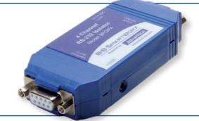
Model BB-9POP4 isolates and protects RS-232 equipment from lightning surges, accidental high voltage shorts and ground loops. RS-232 data signals TD, RD, RTS, and CTS support up to 230.4 kbps. Isolation circuits are 2.5 kV rated and protects valuable equipment while maintaining maximum uptime.
