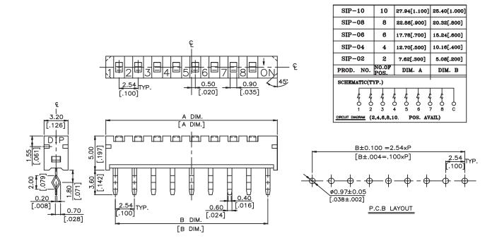
General Tolerance : ±0.2mm Dimensions : Millimetres (Inches)
