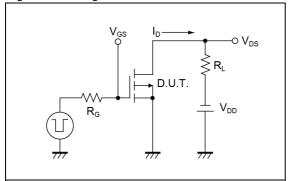
Fig.2-1 Gate Charge Measurement Circuit
