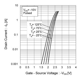
Fig.9 Gate Threshold Voltage vs.
