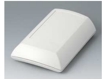
B7010207 ERGO-CASE M, flach ABS (UL 94 HB) grauweiß RAL 9002 150x100x40mm IP 54 opt.
