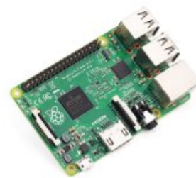
Raspberry Pi 2 Model B w/ ARMv7 Quad Core 1GB RAM ( http://www.seeedstudio.com/depot/Raspberry-Pi-2-Model-B-w-ARMv7-Quad-Core-1GB-RAM-p-2289.html?ref=staffPicked ) SKU: 102110011
