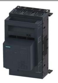
FUSE-SWITCH-DISCONNECTOR 3-POLE, NH00, 160A 60MM BUSBAR SYSTEM COVER LEVEL 32/70 MM BOX TERMINAL FUSE MONITORING ELECTRONIC, EFM 10
