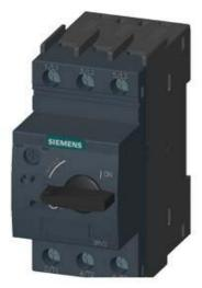
SPECIAL TYPE CIRCUIT BREAKER SIZE S00, FOR MOTOR PROTECTION, CLASS 10, A TRIP.1.1 TO 1.6A,N TRIP. 21A, SCREW TERMINAL, STANDARD SWITCHING CAPACITY AMBIENT TEMPERATURE - 50 DEG. C 500 OPERATING CYCLES
