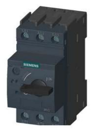
CIRCUIT-BREAKER SZ S00, FOR MOTOR PROTECTION, CLASS 10, A-RELEASE 10...16A, N-RELEASE 208A, SCREW CONNECTION, STANDARD SW. CAPACITY
