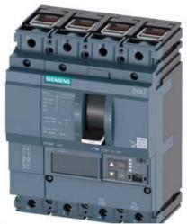
CIRCUIT BREAKER 3VA2 IEC FRAME 100 BREAKING CAPACITY CLASS L ICU=150KA @ 415 V 4POLE, LINE PROTECTION ETU860, LSIG, IN=100A OVERLOAD PROTECTION IR=40A ...100A SHORT CIRCUIT PROTECTION ISD=0,6..10X IN, II=1,5..12X IN NEUTRAL PROTECTION ADJUSTABLE (OFF, UPTO 100%) GROUNDFAULT, SWITCHABLE IG=0,2... 1 X IN, TG=0,050,8MS CABLE CONNECTION
