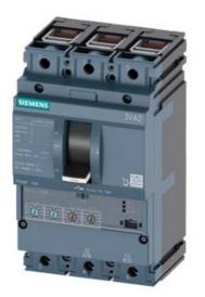
CIRCUIT BREAKER 3VA2 IEC FRAME 160 BREAKING CAPACITY CLASS H ICU=85KA @ 415 V 3POLE, LINE PROTECTION ETU350, LSI, IN=63A OVERLOAD PROTECTION IR=25A ...63A SHORT CIRCUIT PROTECTION ISD=1,5... 10 X IR, II=12 X IN CABLE CONNECTION
