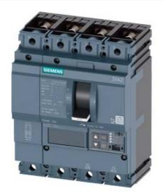
CIRCUIT BREAKER 3VA2 IEC FRAME 250 BREAKING CAPACITY CLASS C ICU=110KA @ 415 V 4POLE, LINE PROTECTION ETU560, LSIG, IN=160A OVERLOAD PROTECTION IR=64A ...160A SHORT CIRCUIT PROTECTION ISD=0,6..10X IN, II=1,5..12X IN NEUTRAL PROTECTION ADJUSTABLE (OFF, UPTO 160%) GROUNDFAULT, SWITCHABLE IG=0,2... 1 X IN, TG=0,050,8MS BUSBAR CONNECTION
