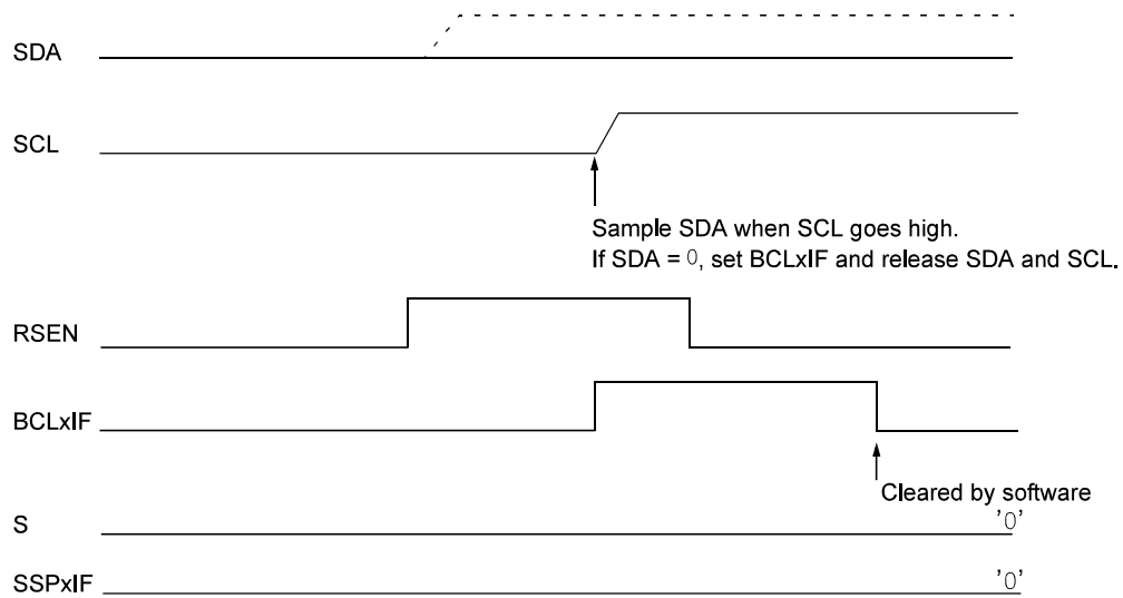
Figure 29-37. Bus Collision During a Repeated Start Condition (Case 1)
