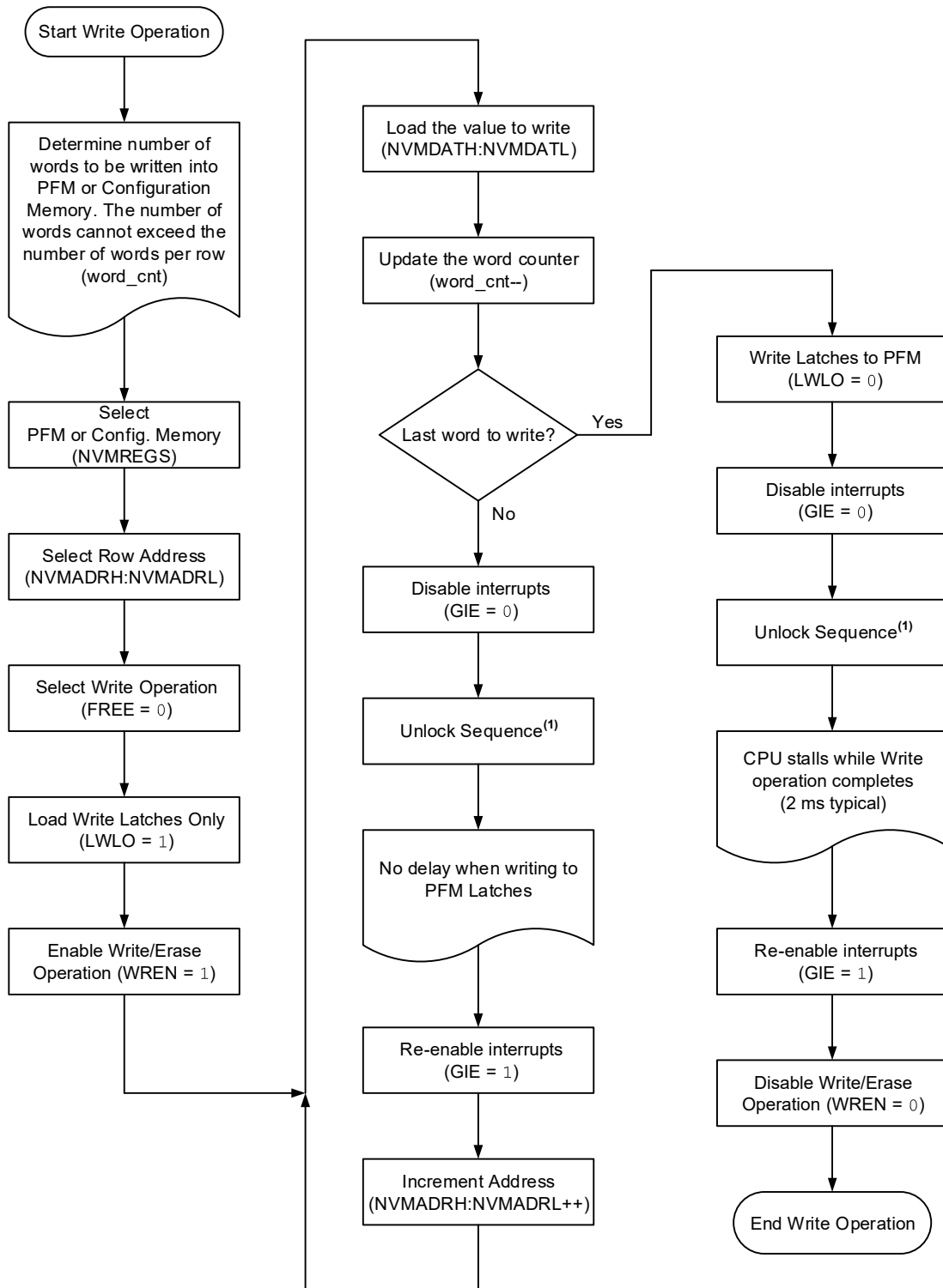
Figure 15-5. Program Flash Memory Write Sequence
