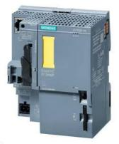
SIPLUS ET 200SP CPU 1512SP F-1 PN rail based on 6ES7512-1SK01-0AB0 with conformal coating, -40...+70 °C, OT4 with ST1/2 (+85 °C for 10 minutes), no pluggable BusAdapter, central processing unit with work memory 300 KB for program and 1 MB for data, 1st interface, PROFINET IRT with 3-port switch, 48 ns bit performance, SIMATIC Memory Card required,
