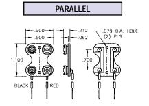
Contacts: Steel, Nickel Plate Wire: #22 AWG, 7/30 Prebond End Strip: .375 Long, Tinned
