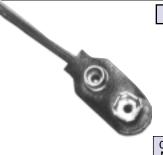
Cover Sizes:  $1.125 \times .530$ Contacts: Phos. Br., Nickel Plate Wire: #26 AWG, 7/34 End Strip: .250 Long, Tinned
