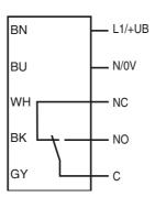
The relay-functions "NC" and "NO" bear on the switching mode "Dark-ON". This complies to the default setting of the light/dark switch (factory setting).
