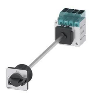
Switch disconnector 3LD3, main switch 3-polig + N, lu 32A operational switch at AC-23 A at 400 V 11,5 kW floor mounting Base mounting with door coupling center-hole 22,5 mm knob-operated mechanism black 48 x 48 mm with auxiliary 1NO+1NC
