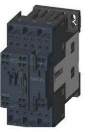
CONTACTOR, AC-3, 7.5KW/400V, 1NO+1NC, AC 230V 50HZ, 3POLE, SZ. S0 SPRING-LOADED TERMINAL FOR UPRIGHT MOUNTING POSITION
